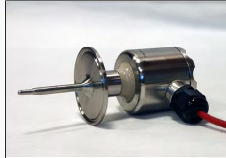
Once mounted, the RTC-168 combines the external cable reference sensor and the built-in internal reference sensor to fuel its dual-zone technology and proven Set Follows True function to ensure consistent temperature from the main zone through the upper calibration zone. As technicians can easily transport the RTC-168, they can now provide in-field calibration of difficult sanitary sensors.
